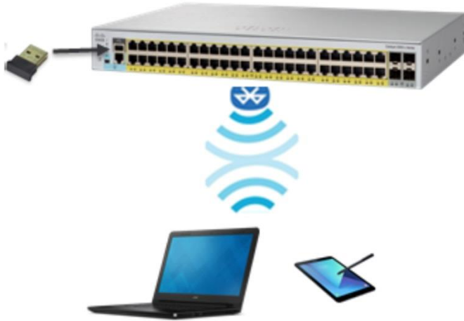
Figure 4. Over-the-air switch access using Bluetooth
