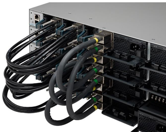
Figure 9. StackWise-480 and StackPower connectors
